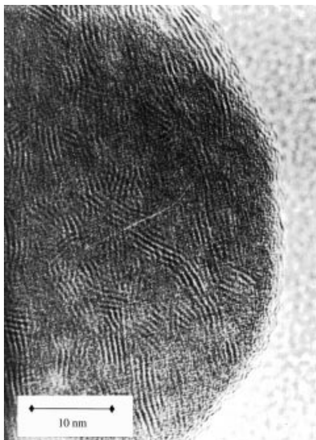
Figure 4. HREM image of the sample treated with \text{H}_2\text{S} at 873 K for 8 h.
